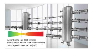
Air volume standard calibration system Air volume: 0.5 m<sup>3</sup>/h ... 1000 m<sup>3</sup>/h
